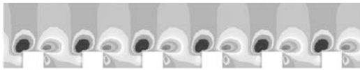
Fig. 2(b) v velocity contour on yz plane with uniform roughness height and pitch
